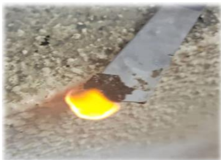
Figure 6: Burn test result of FR4 bioplastic films
